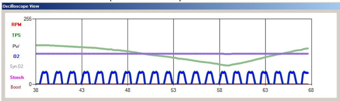
Similarly all the important parameters can be logged to a file while in operation by ticking the "LOG" check box. This will ask for a file name, and then stream data from the Power Strecher continuously into the file. If a wide band O2 sensor (AFR sensor) is used, it can be read simultaneously for off line "auto tuning".
