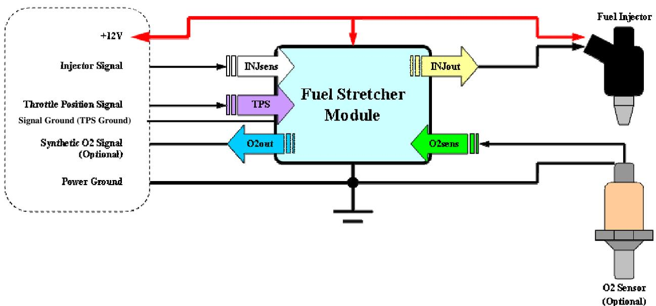
For multi-cylinder engines the Injector sense line and Injector control (Inj out) are the same color (eg. Both are yellow). The thick wire is always the injector out line (as it carries the current from the injector), and the sense line is the thin wire.
